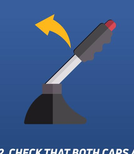
2. CHECK THAT BOTH CARS ARE IN NEUTRAL WITH THE HANDBRAKES ON.
