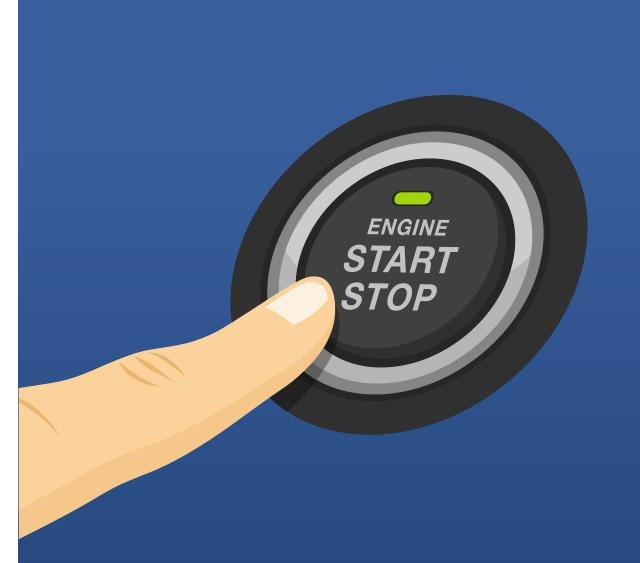
6. START THE ENGINE OF THE CAR WITH THE CHARGED BATTERY. LET IT RUN FOR A MINUTE.
