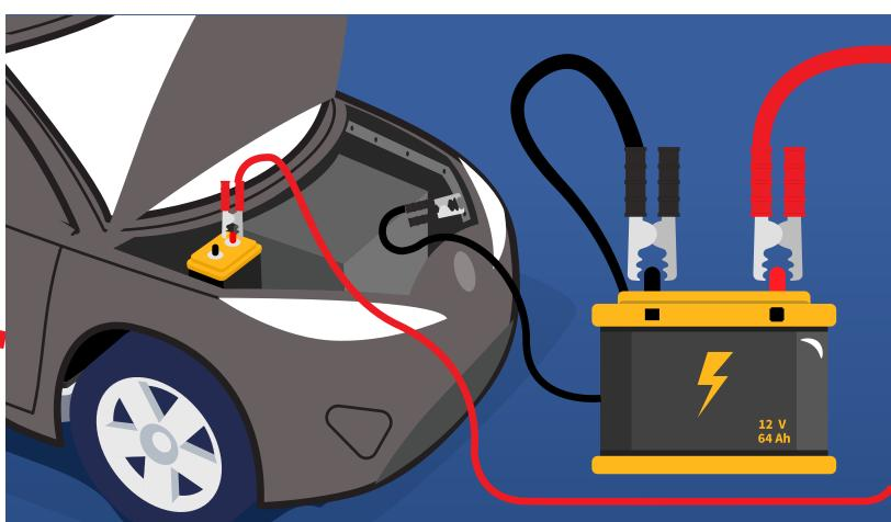
4. ATTACH THE BLACK JUMP LEAD TO THE NEGATIVE TERMINAL OF THE CHARGED BATTERY, THEN CLIP THE OTHER END TO ANY UNPAINTED METAL BRACKET ON THE CAR WITH THE FLAT BATTERY.
